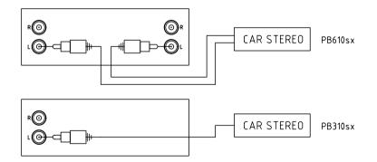
CAR SIGNAL INPUT (RCA LINE OUT) MUST BE CONNECTED TO ONLY EACH "L" CHANNEL (BRIDG SWITCH KNOB SHOULD BE SELECTED MO). IF CAR SIGNAL INPUT IS CONNECTED TO "R" CHANNEL THERE SHALL BE NO POWER OUT (NO SOUND).
